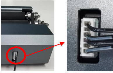
Connect to the Rotary
